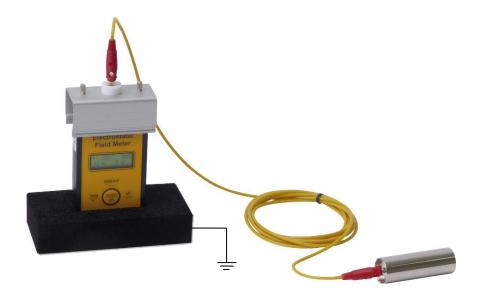
Important: Only voltage up to 4 kV can be measured!
