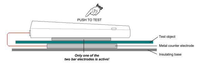
Measurement of the point-to-point-resistance R<sub>p-p</sub>
